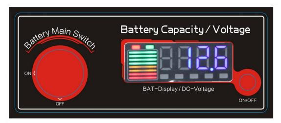
When the voltage of battery is 13.0 volt or above, BAT-Display is full, which doesn't mean the battery charged 100% fully. Please charge the battery immediately, when BAT-Display goes down to red sector, or the voltage is 11.0V or less.
